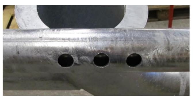
If this does not help, the cover tube is most likely full of dried manure. Release the set screws on the cover tube.
