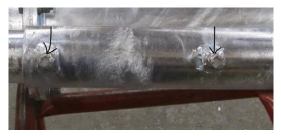
Loosen the cover tube from the pump housing and from the gearbox housing. Rinse cleanly inside the cover tube.
